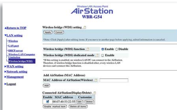
Figure 4.1.6b Wireless Bridge (WDS) Settings
