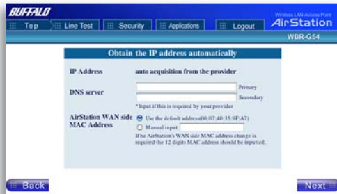
Figure 3.5.2b Auto IP/ Manual DNS Settings
