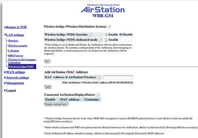
Figure 4.1.6 Wireless Bridge (WDS) Settings
