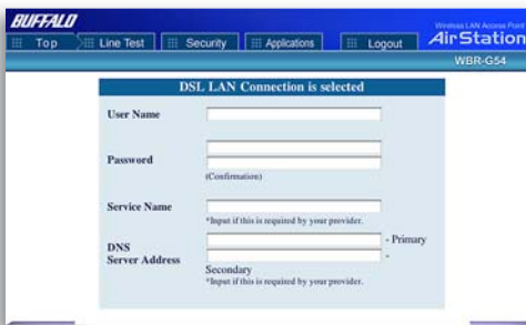
Figure 3.5.1b DSL PPPoE Settings Screen
